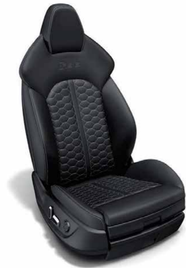
RS sport seats, front with shaped seat side bolsters for better lateral support, integrated head restraints and RS 6 embossing on the front-seat backrests; manual adjustment of seat height, fore/aft position, seat angle, backrest angle and belt height; electric 4-way lumbar support; extendable thigh support. (The image shows RS sport seat, front, electrically adjustable, in Valcona leather, black with honeycomb pattern in rock grey.)
