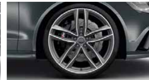
Cast aluminium wheels in 5-twin-spoke design in matt titanium look, gloss turned finish size 9.5 J x 21 with 285/30 R 21 tyres*
