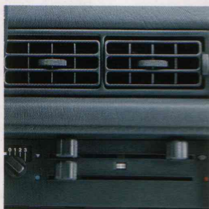
Heating and ventilation system with 3-speed fan.
