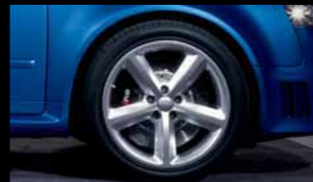
Cast aluminium wheels in 5 spoke styling, size 8.5 J x 18 with 255/40 R 18 tyres
