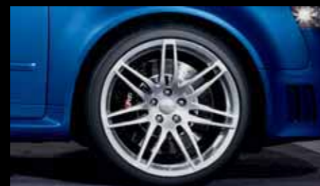
Cast aluminium wheels in 7 double-spoke styling, size 9 J x 19 with 255/35 R 19 tyres
