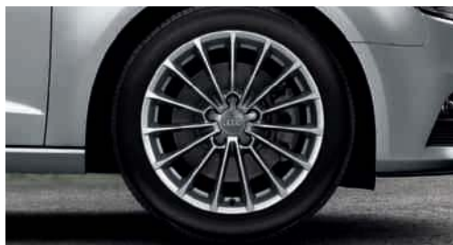
Cast aluminium wheels in 15-spoke design size 7.5 J x 17 with 225/45 R 17 tyres (optionally available with run-flat tyres)
