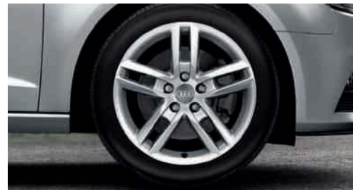
Audi exclusive cast aluminium wheels in 5-twin-spoke design size 7.5 J x 17 with 225/45 R 17 tyres. From quattro GmbH
