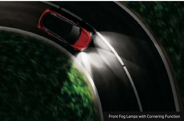
Front Fog Lamps with Cornering Function
