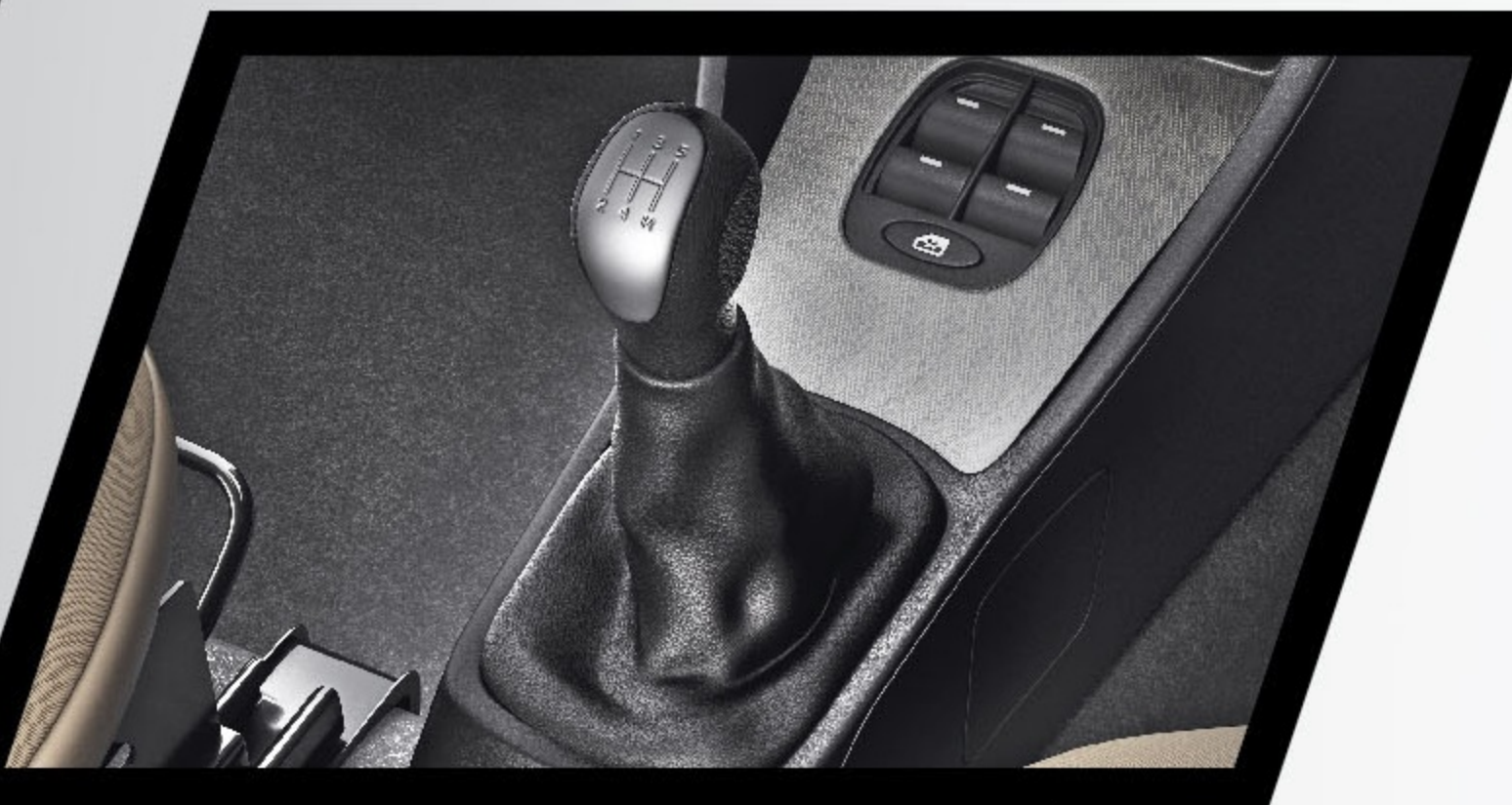
F-shift Gearbox (TA 65* Cable-shift)
