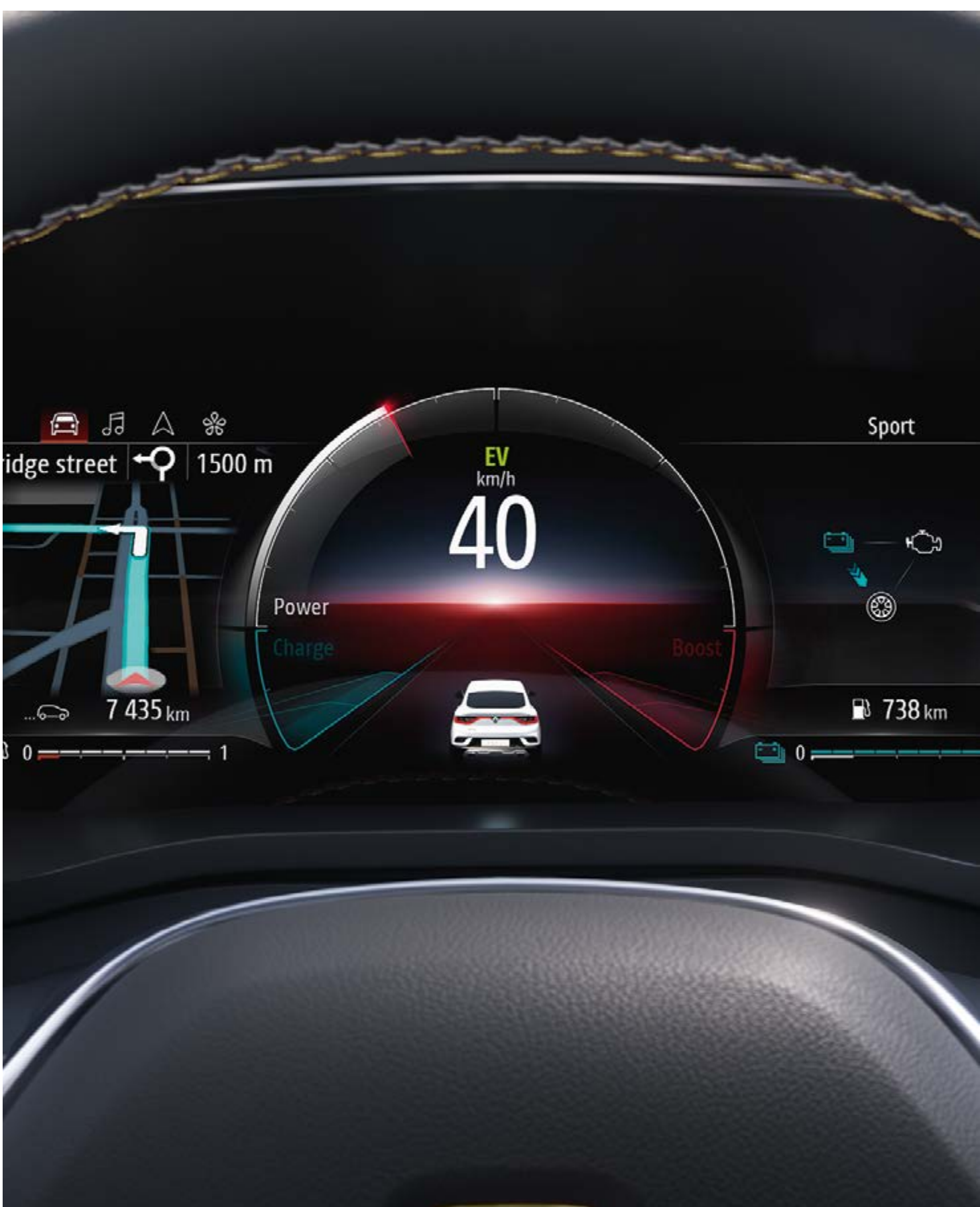
10" digital instrument panel (1) with driving information
