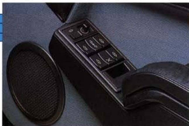
Renault 25 V6 Turbo: Driver's armrest controls
