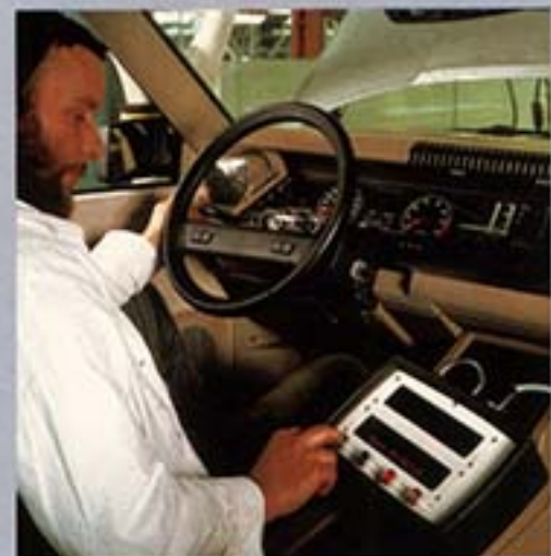
Programmed electrical checks
