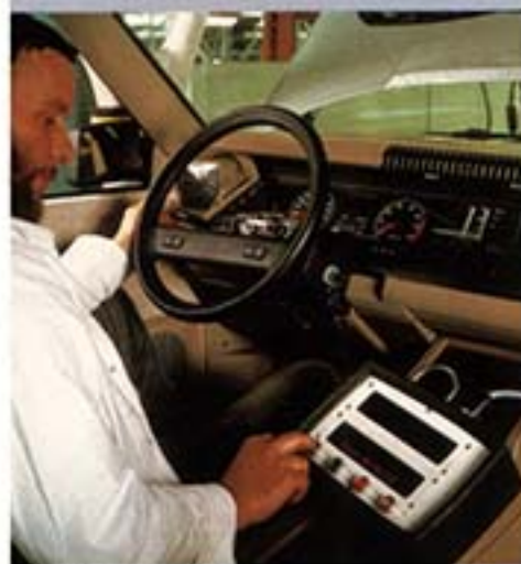
Programmed electrical checks
