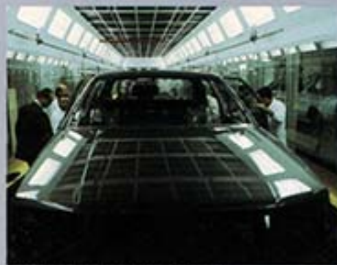
Checking of sealing before fitting out
