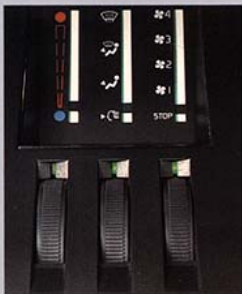
Heater control unit.
