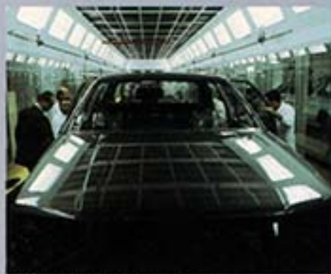
Checking of sealing before fitting out
