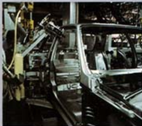
Measuring dimensions for door assembly by robot
