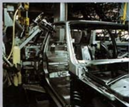
Measuring dimensions for door assembly by robot
