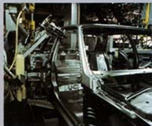
Measuring dimensions for door assembly by robot
