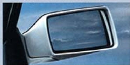
Electrically operated and heated door mirror.
