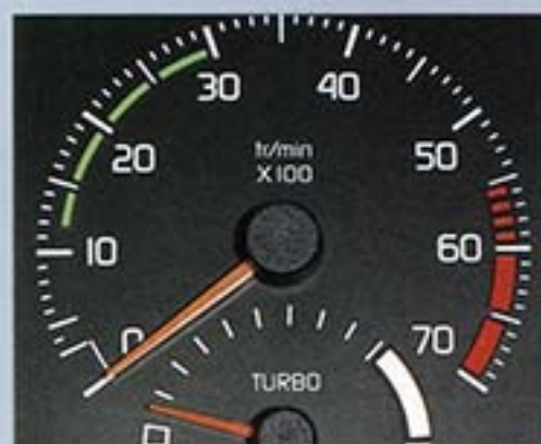
Renault 25 V6 Turbo rev. counter incorporating Turbo gauge.
