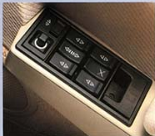
Control panel on driver's armrest.
