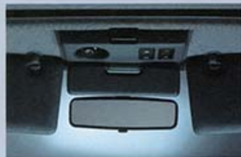
Aircraft type swivel interior light on roof console and central sun visor.
