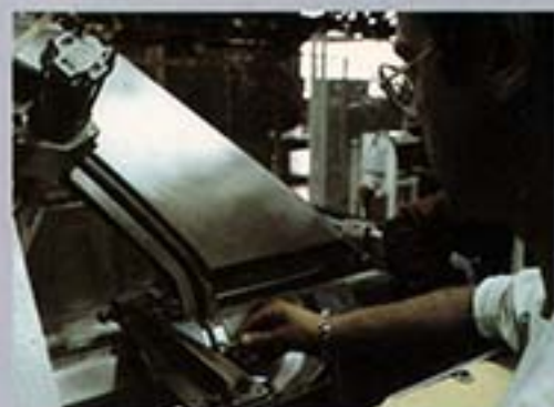
Checking of tolerances at 90 different points
