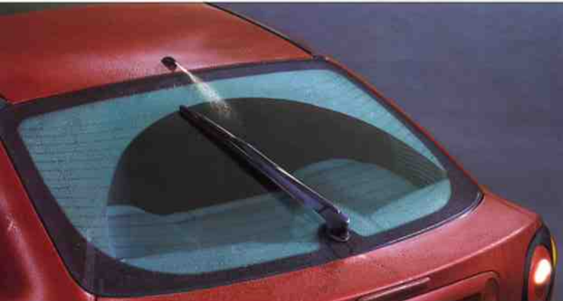
Rear wash-wipe gives single automatic sweep when reverse is engaged with optional Electrics Pack.
