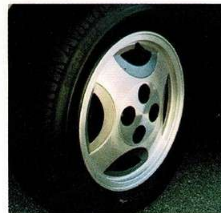
Cast Aluminum Styled Wheels With Michelin TRX Tires.
