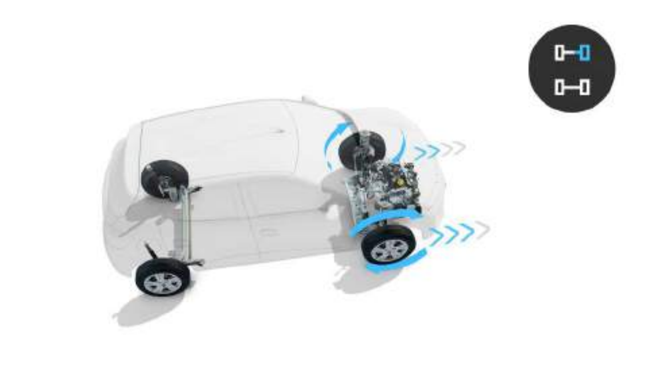
traction control system Limits wheel slip during starting, acceleration and braking.
