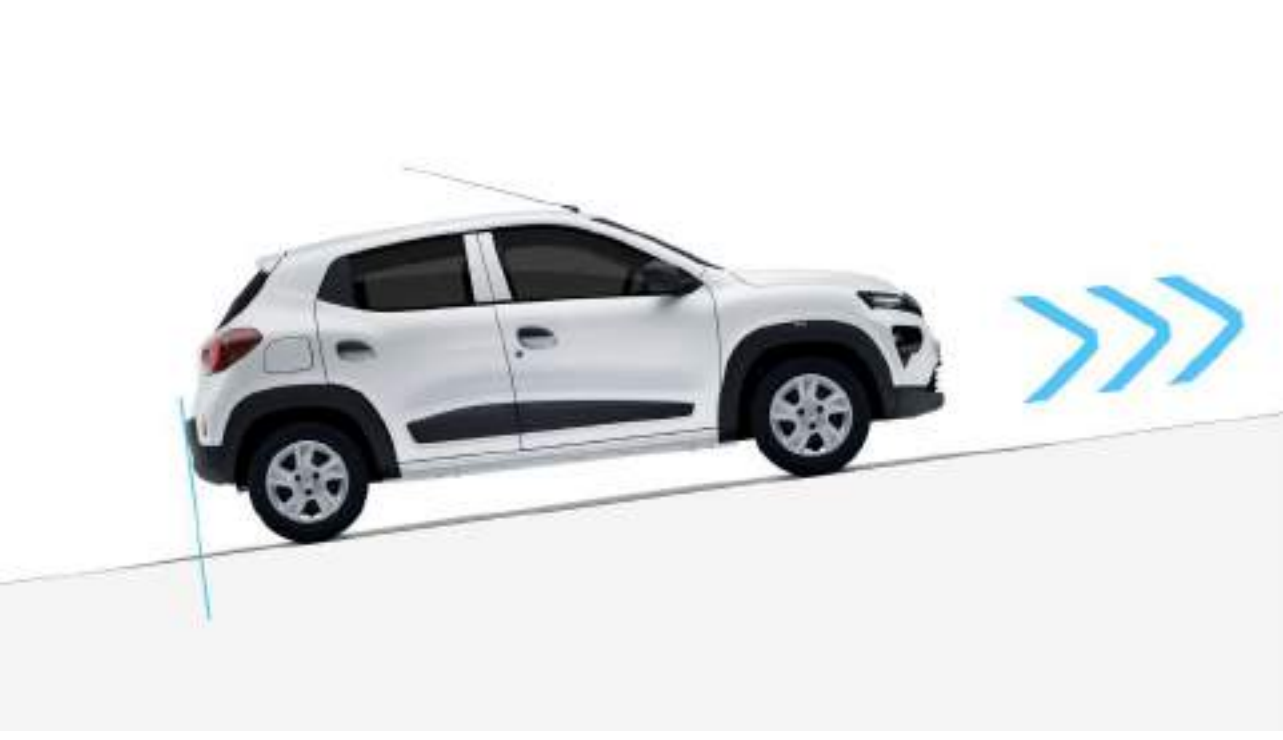
hill start assist 2 Maintains brake pressure for two seconds, preventing rollback when you move away on a steep slope.
