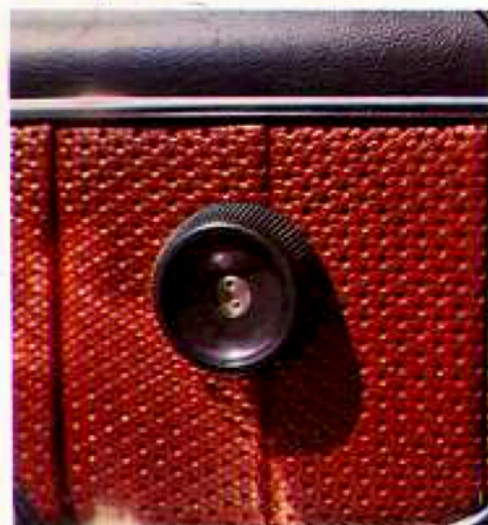
New revolving knob for regulation of draught deflectors.
