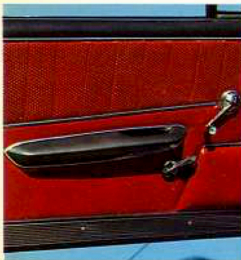
New inserts on inner door panels. Inner door handles below armrest.
