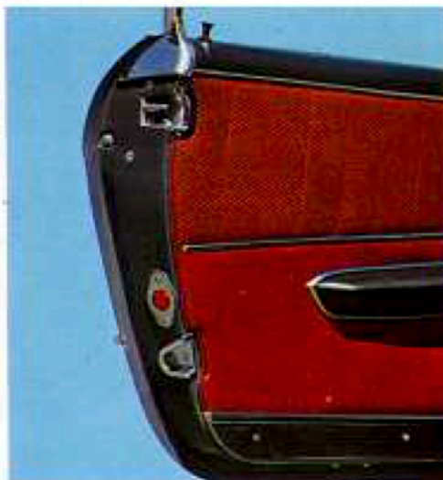
New designed door locks. Warning red light when door is open.
