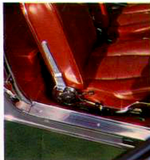
Device for back-rest locking of front seats. Door sill plate.
