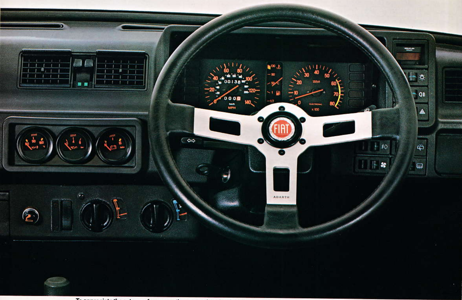
To appreciate the extra performance, the comprehensive dashboard includes rev counter, voltmeter, oil temperature and pressure gauges.
