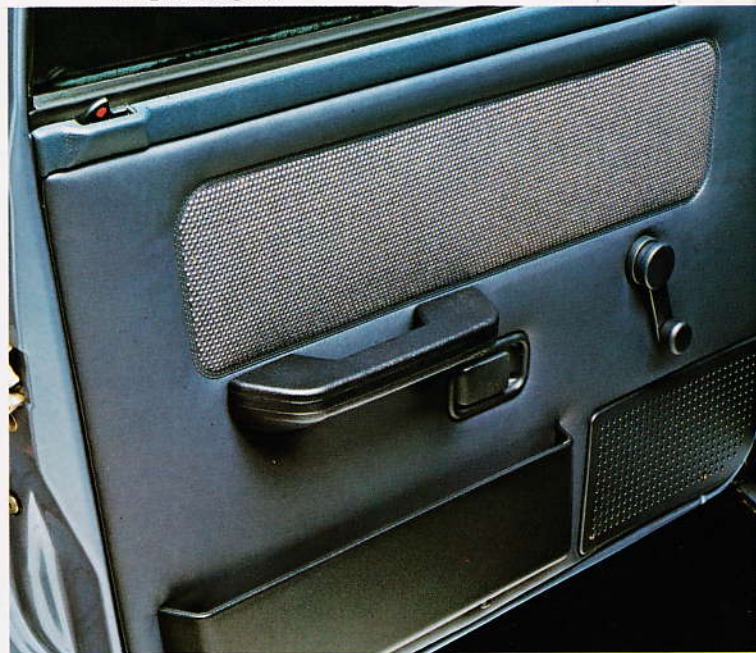
The doors now carry the seat cloth material as well as deep pockets and speakers.
