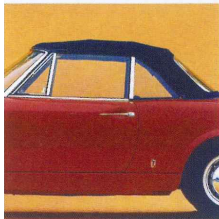
Easily manoeuvrable folding top. Wide rear light. Rear quarter window glasses which drop away when the top is folded down.
