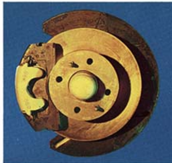
Disc brakes on all four wheels plus braking effort distribution valve.
