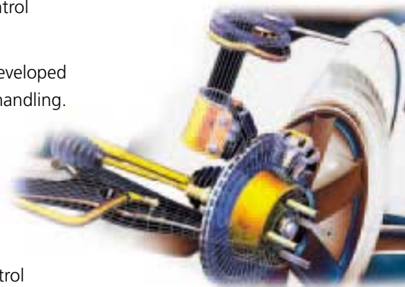
Independent front McPherson strut for superior ride and handling
