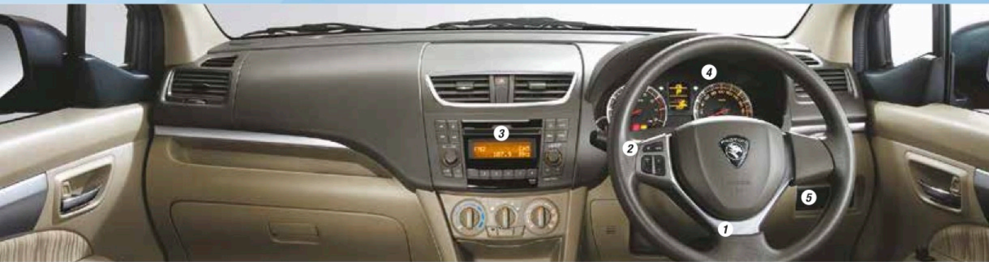
1 Electric Power Steering 2 Steering Audio Switches* 3 2-DIN Radio 4 High Grade Meter Cluster 5 Headlamp Levelling
