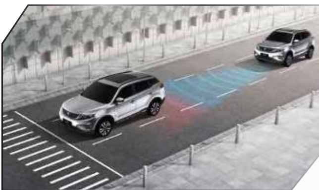
Autonomous Emergency Braking (AEB) and Forward Collision Warning (FCW)
