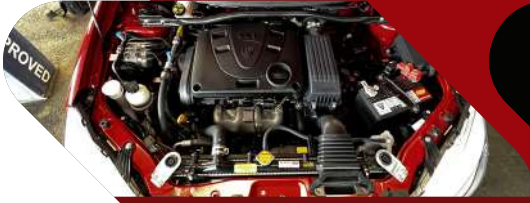
1.3L, 4 Cylinders In-Line, 16 Valve DOHC, VVT Engine
