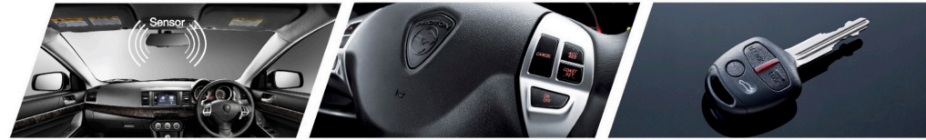
The rain sensor triggers the windshield wipers when there is rain. The auto light sensor automatically turns on your headlights when the lights are low.
