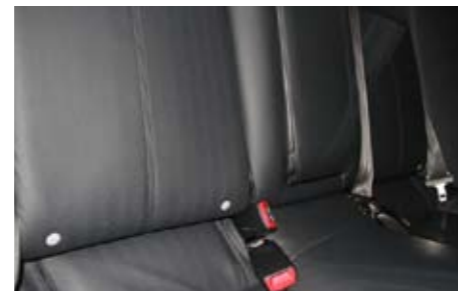
The Proton INSPIRA has ISOFIX mounting points for child seats to ensure the safety of children passengers.
