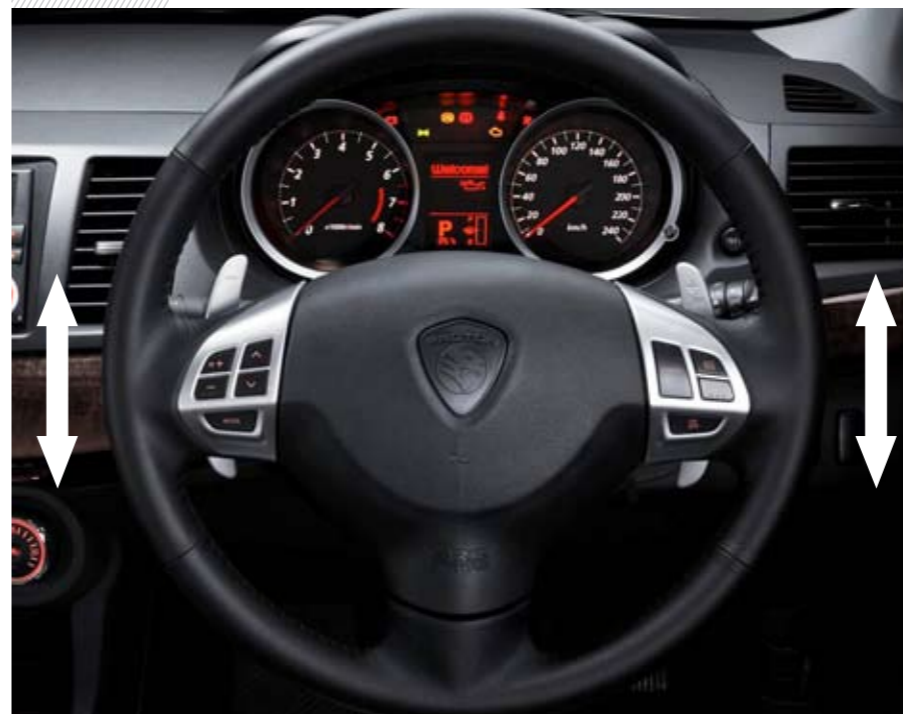
The adjustable tilt steering enables you to sit comfortably in the driver's seat as you are driving.
