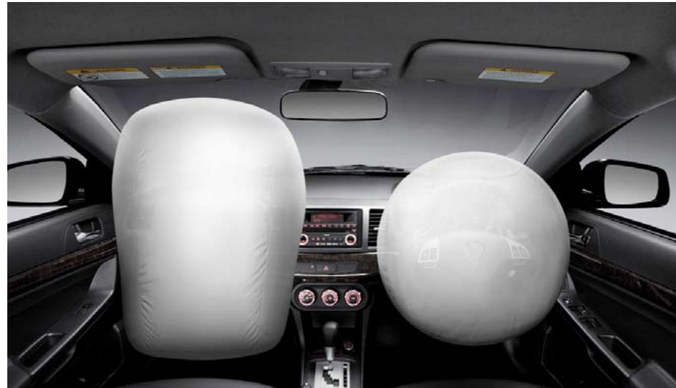
Dual SRS Airbags Protects both driver and front passenger from severe injuries in the event of a collision. It also helps to slow down head and chest movement during a sudden crash.
