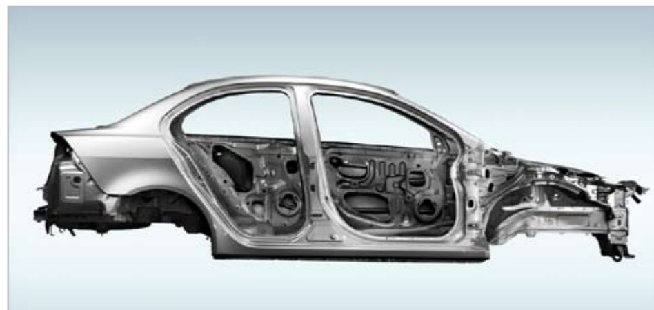
Strong Body Structure The RISE (Reinforced Impact Safety Evolution) body is designed to protect passengers by using extensive front and rear crumple zones to absorb impact energy.
