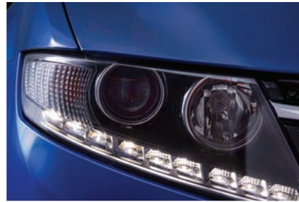
LED daytime running lights come on automatically when you start the car.
