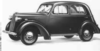
1937 – The Vauxhall 'H'-type, the first British car to have integral construction.
