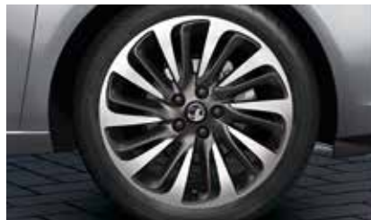
18-inch 10-spoke alloy wheels with 225/40 R 18 tyres.
