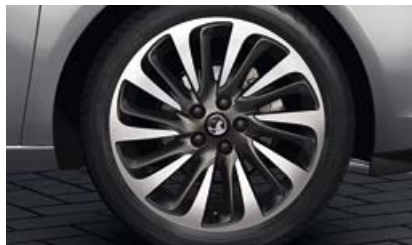
18-inch 10-spoke alloy wheels with 225/40 R 18 tyres.
