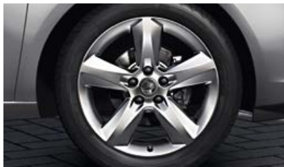
17-inch five-spoke alloy wheels with 225/45 R 17 tyres.
